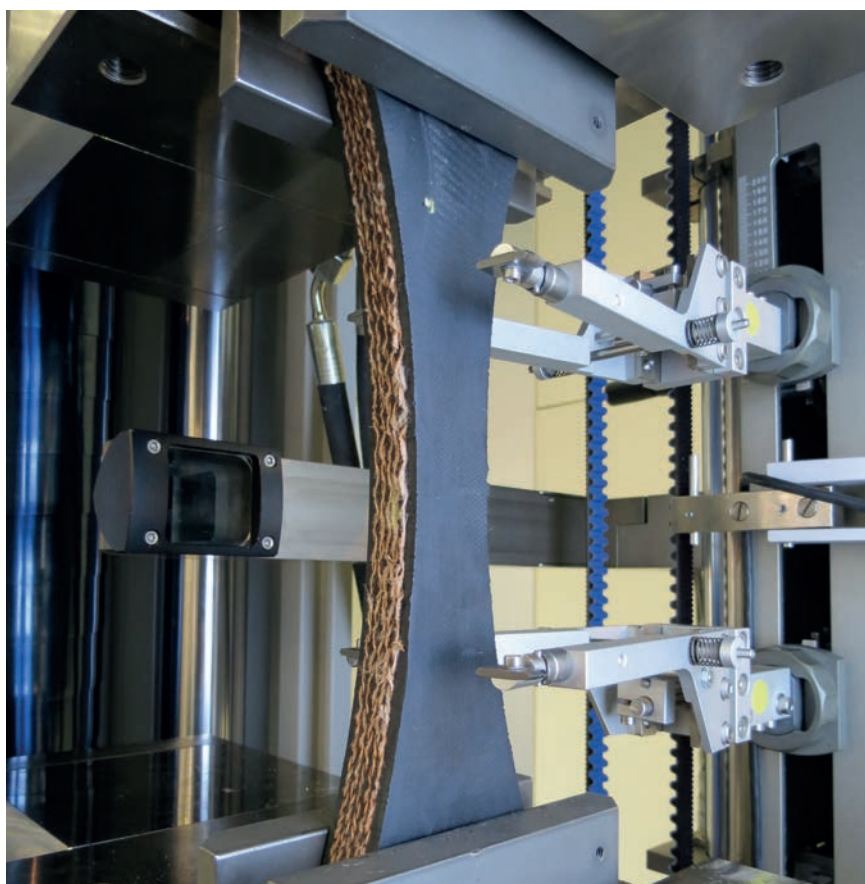
Fig. 1. Tensile test on conveyor belt
