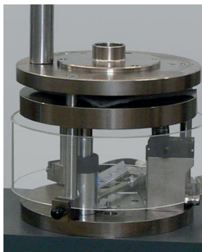
Fig. 2. Static puncture test (CBR test)
