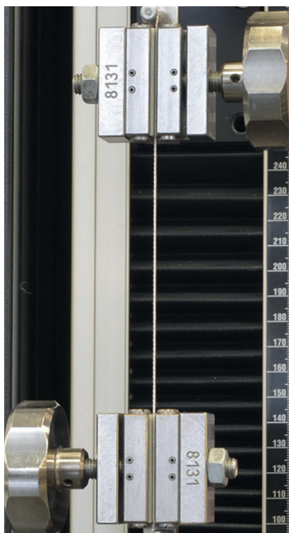
Fig. 1. Tensile test on sewing yarn
