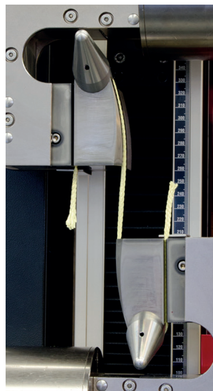
Fig. 2. Tensile test on aramid yarn
