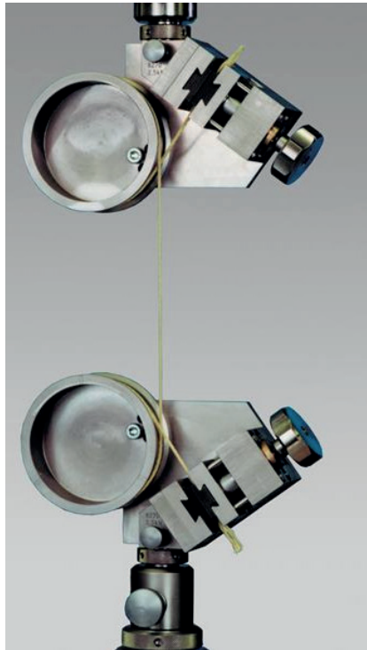
Fig.1. Tensile test on multi-filament yarn
