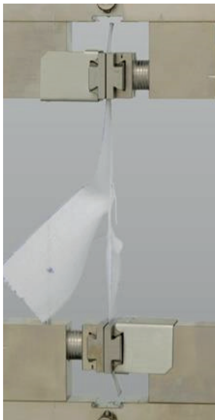
Fig. 1. Tear growth test on textiles
